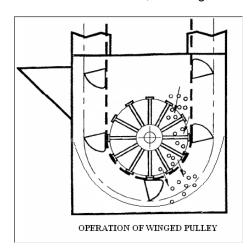
**Boot Pulley** – Most boot pulleys for grain are smooth surfaced, but for sticky meals which build up on the inside of the belt and cause belt stretch as well as other belt issues; a wing type pulley is best as it allows the surplus material to fall through the wings instead of building up between the pulley and the belt. A wing type pulley also reduces damage to pellets.
