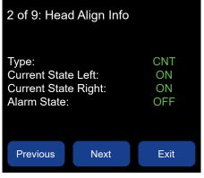
Image 8B Head Align Info - Contact Sensor
