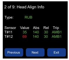
Image 8C Head Align Info - Rub Block Sensor
