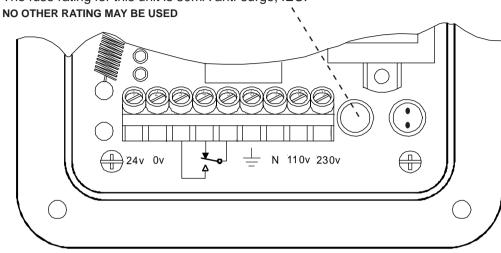
Warning: All wiring must be in accordance with local and national electrical codes and should be undertaken by a qualified electrician.
