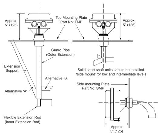
Extension Rods and Guard Pipes can be provided for low level or when RTS's are mounted high in bin/silo roof
