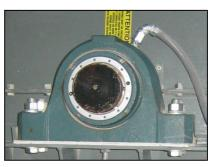
Sensor Installed on Conveyor Bearing
