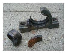
**Example of Bearing Failure**
