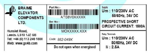
SUBSTITUTE X'S IN PART NO. WITH FULL PRODUCT PART NUMBER SUBSTITUTE X'S IN SERIAL NO.WITH MANUFACTURING BATCH NUMBER SUBSTITUTE X IN CODE WITH MANUFACTURE ISSUE STATUS Alternative 4B Components label part 1
