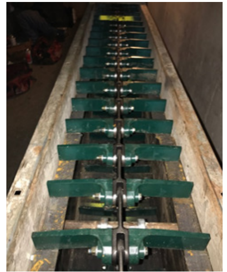
Bolt-N-Go Chain shown with green nylon paddles for color sorter detection
