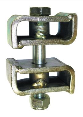
The **Supergrip** belt fastener secures belting on bucket elevators. The two ends of the belt are gripped between extruded steel plates, clamped together by zinc plated high tensile bolts and self-locking nuts.
