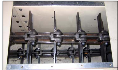
Bolt 'N' Go System Drop Forged Chain Application on a Conveyor
